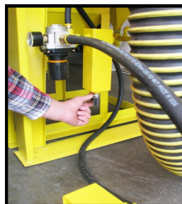
Air regulator with pressure booster and moisture separator
