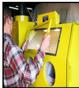
Safe & Easy window frame removal to replace inside glass
